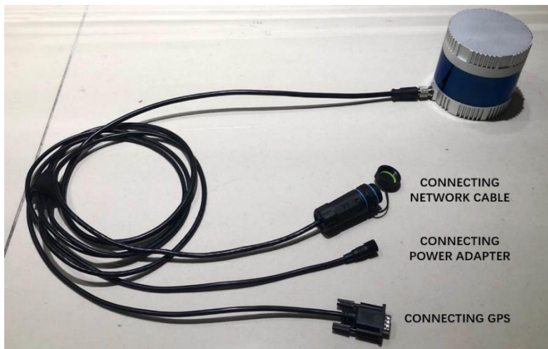
Figure 3.1 Connecting Lidar and Computer
